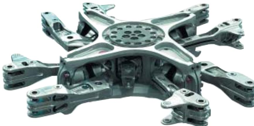
*Designed to flaw tolerant certification requirements, the unlimited life S-92 main rotor head features redundant load paths and elastomeric bearings. The result is 50,000 hours before overhaul.*
