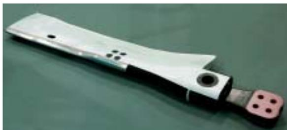
*Bearingless composite flexbeam tail rotor design is bird strike certified*
