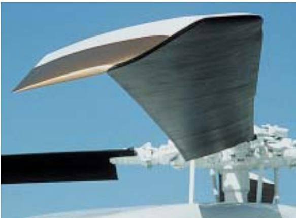
*Unlimited life main rotor blade incorporates composite spar technology and utilizes a swept, tapered anhedral tip. This design provides improved lift and maneuverability.*
