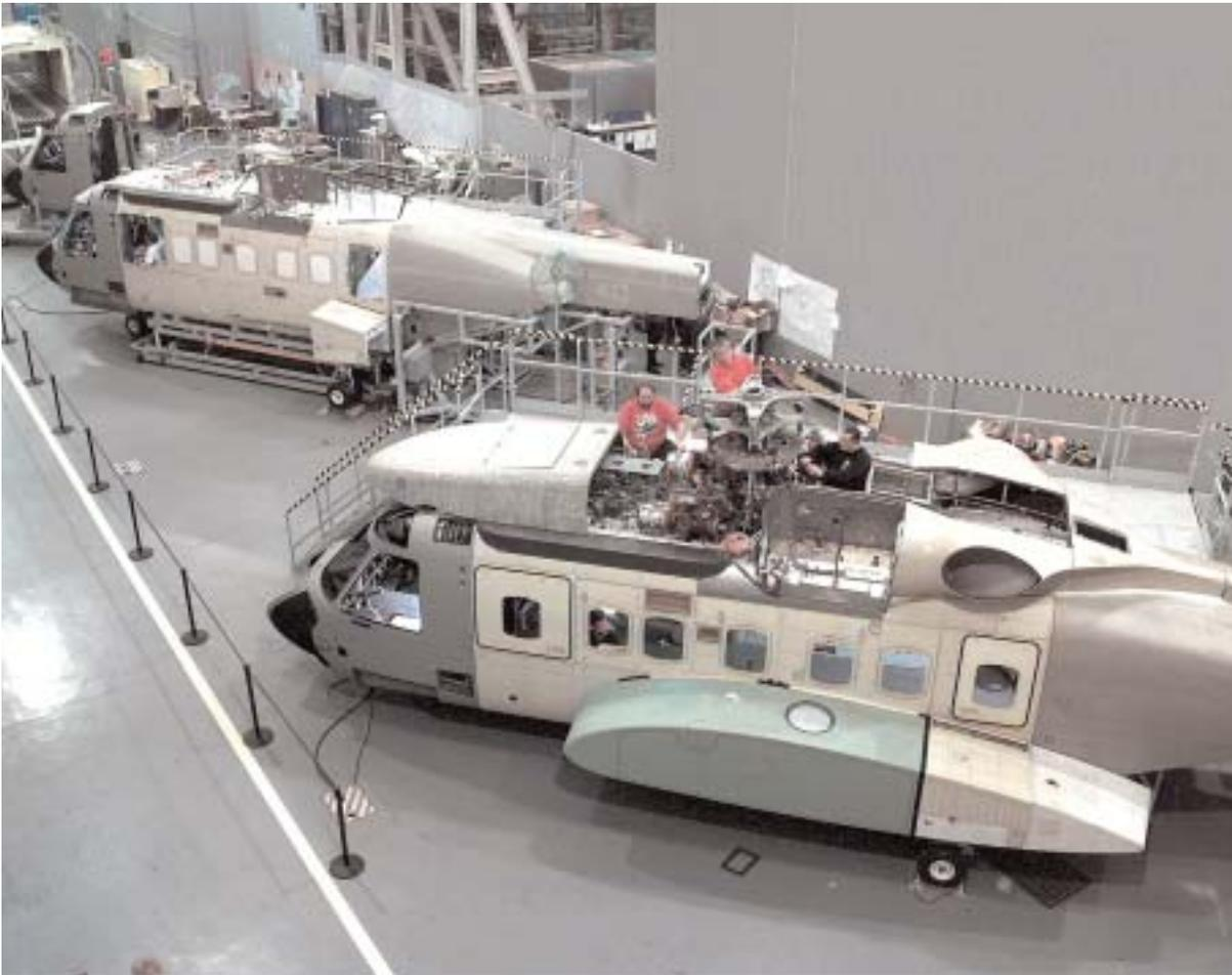
*Parts manufactured by worldwide partners come together on the S-92 assembly line at Sikorsky's Stratford, Connecticut facility.*
