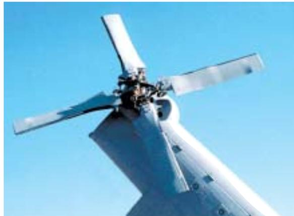
*Anti-torque control is provided by unlimited life tail rotor blades with bearingless composite flexbeam. The pitch control links use elastomeric bearings.*
