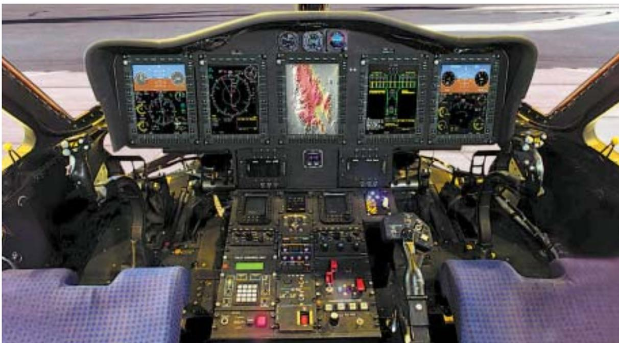
The S-92 cockpit and display panel, shown here with an optional fifth liquid crystal, multi-function display.
